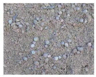
Boughton IN 1 intensive green roof substrate has been designed to contain a greater proportion of organic matter and finer sand particles.
