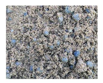
10 Clay (<0.002 mm) Silt (0.002-0.063 mm) 6 Sand (0.063-2.0mm) 84 Texture Class (UK cl) LS Stones (2-20mm) 1.9 Stones (20-50mm) 1.1 0 Stones (>50mm) 8.2 pH Value (1:2.5 water extract) **Organic Matter** 1.4
