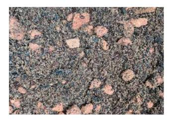
Boughton BLMP SuDs Soil is a multi purpose blend of sand, PAS 100 green waste compost, crushed brick and coir, designed as a layer for Swales and rain gardens, to support a range of intensive vegetation.
