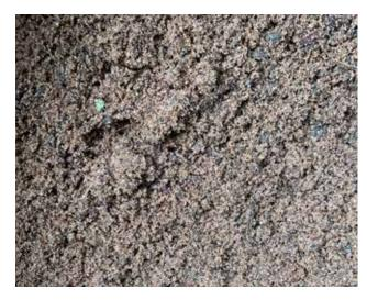
Boughton BLHP High Permeability Soil is designed to be used in shallow swales which border paths (streets and pedestrian).
