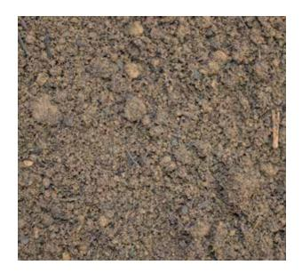
BLS 20 topsoil is processed by passing natural 'As dug' topsoil over modern screening equipment to remove all large lumps/stones and other deleterious materials, such as plant roots and leaves.
